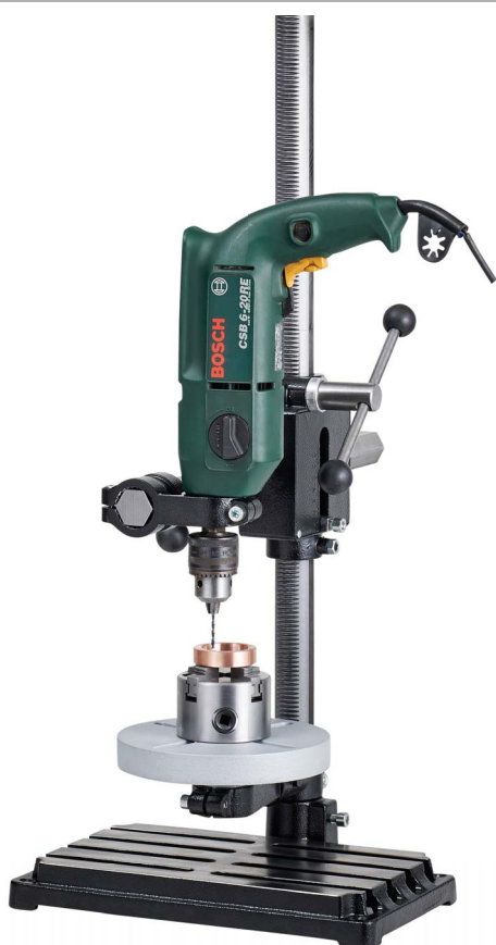
Vertical pitch circle drilling
